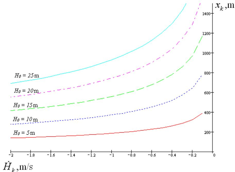
Fig. 1. Flareout distance depending on a vertical velocity of runway tangency for different initial altitudes
