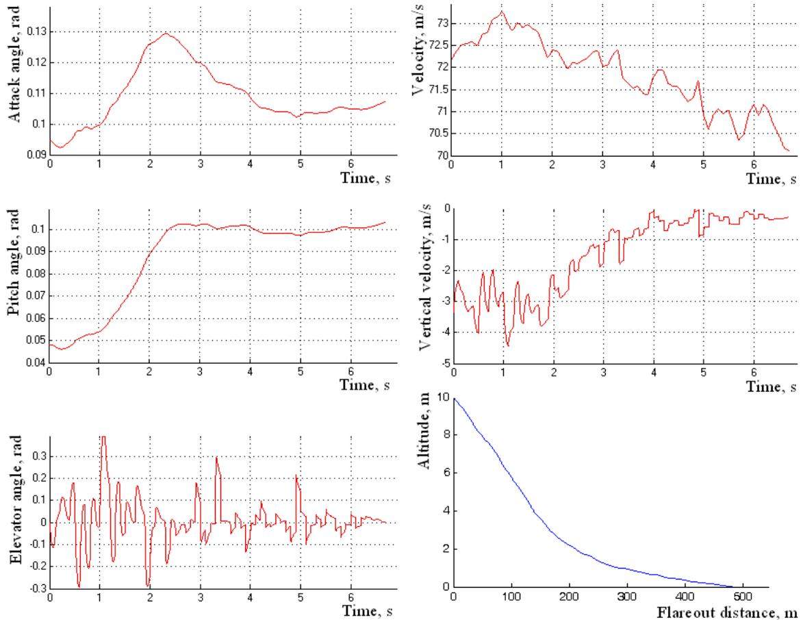
Fig. 2. Flareout of Ty154 in conditions of atmospheric turbulence
