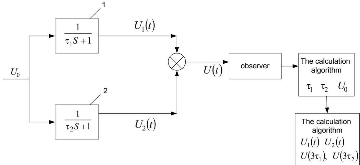
Fig. 1. Block diagram of input signal transforming and processing system
